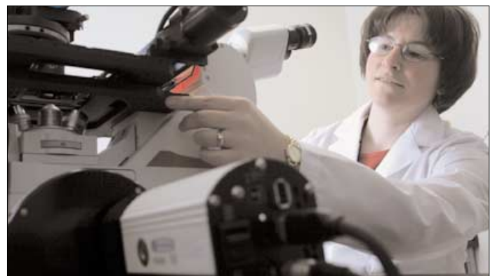
Karen Mossman, a member of the Infectious Disease division of the Centre for Gene Therapeutics, operates a Leica DM-IRE2 inverted fluorescent microscope, which allows researchers to monitor cellular processes in living cells in real time.
